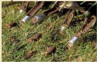
a machine that removes plugs of soil and grass roots. The plugs can be left in place to rot and feed the lawn (or removed if you prefer) and then you should apply a top-dressing of sand, raking it into the holes that have been created, in order to provide good aeration and water drainage.
